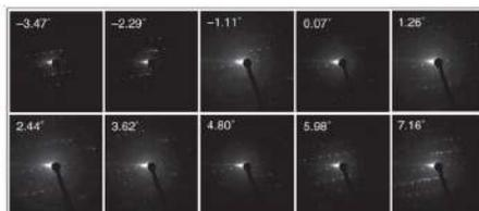
*Selective ED patterns of the 1-Abtistine microcrystal during continuous rotation. The number of each frame represents a starting rotation angle of each ED patterns. The diffraction patterns were obtained every 1.18°*
